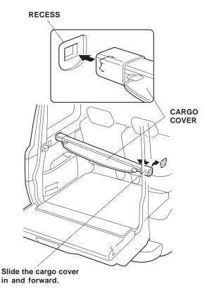
Install the cargo cover into the recess in the left rear side trim panel, then compress the cargo cover, and install it in the recess in the right rear side trim panel.
