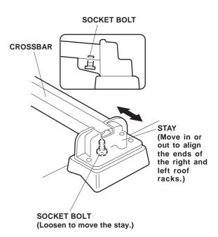
Temporarily tighten the 12 socket bolts and 12 washers.
