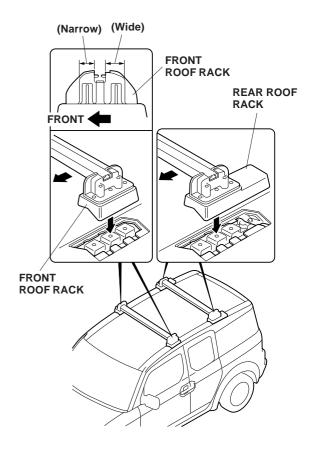
If the ends of the right and left roof racks are not aligned, adjust them by loosening the crossbar socket bolts and moving the stays in or out as necessary.
