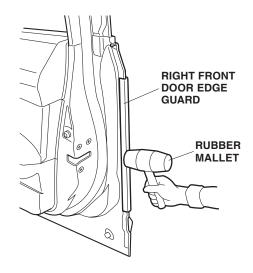
7. Repeat steps 3 through 6 to install the left front door edge guard.
