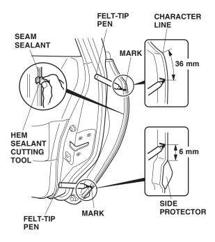
9. Position the hem sealant cutting tool against the door edge, and trim the seam sealant from mark to mark.
