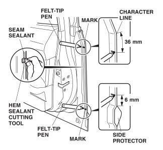
4. Position the hem sealant cutting tool against the door edge, and trim the seam sealant from mark to mark.
