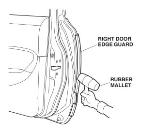
7. Repeat steps 3 thru 6 to install the left door edge guard on the left front door.
