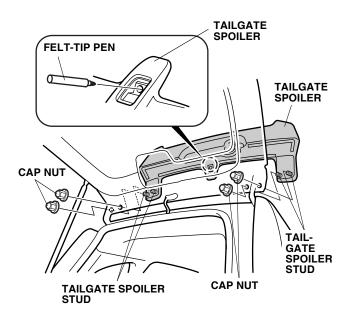
12. Remove the tailgate spoiler, and lightly center-punch the mark you made.
