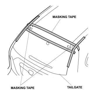
7. Open the tailgate. Apply masking tape over the ends of the tailgath housing. Close the tailgate.
