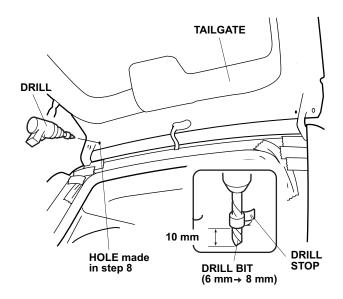
Insert the studs on the tailgate spoiler into the holes you drilled, and loosely install the four cap nuts. Close the tailgate. Using a felt-tip pen, mark the tailgate through the center hole in the spoiler.
