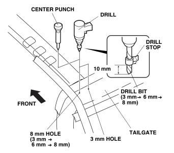
9. Repeat step 8 to drill the tailgate on the right side of the vehicle. Remove any burrs from the edges of the holes using a file, and apply touch-up paint to the edges. Allow the touch-up paint to dry.
