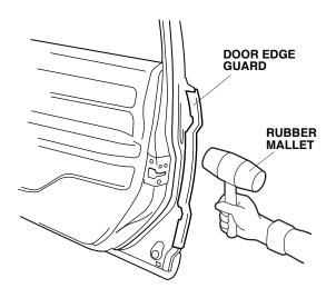
Repeat steps 3 thru 6 to install the left front door edge guard.
