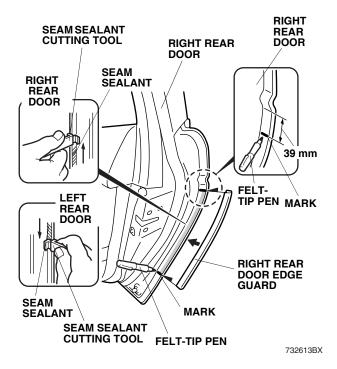
11. Position the cutting edge of the seam sealant cutting tool against the right rear door edge, and trim the seam sealant from mark to mark.
