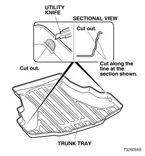
2. Open the trunk lid. Place the trunk tray on the trunk floor.
