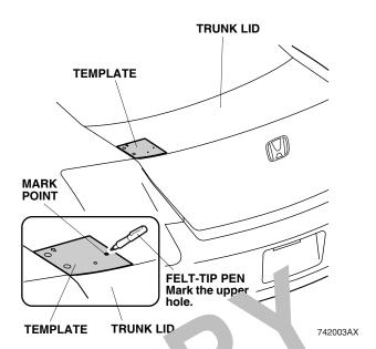
7. Flip the template over. Align the template with the right side trunk lid. Using a felt-tip pen, make two marks on the right side trunk lid as shown. Remove the template.
