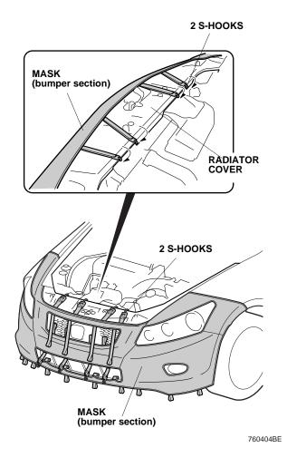
13. Route the upper strap of the mask through the inside of the front grille as shown. Then route the upper strap of the mask through the loop on the lower strap of the mask as shown. Repeat on the three other straps.
