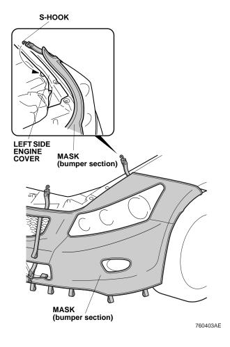
12. Attach two S-hooks to the bottom edge of the radiator cover.
