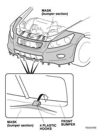
16. Route the elastic cord through the 12 loops on the bottom of the mask. Attach an S-hook to the hole of the inner fender as shown. Attach the other S- hook to the hole of the inner fender to the other side.
