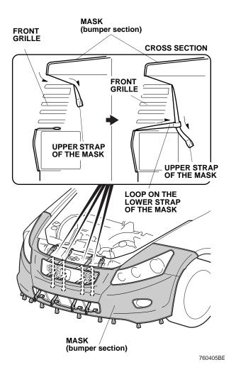
14. Continue routing the upper strap of the mask through the inside of the front bumper and attach the S-hook to the loop on the upper strap of the mask as shown. Repeat on the other straps.
