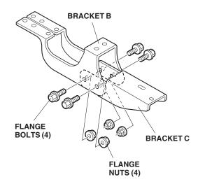
Assemble two rear bracket assemblies using brackets A and C along with four flange bolts and four flange nuts. Leave the nuts and bolts loose at this time.
