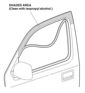
3. Locate the door sash in the area where the EPT sealer will attach. Using isopropyl alcohol on a shop towel, thoroughly clean the area.
