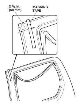
12. Using isopropyl alcohol on a shop towel, clean the shaded area of the door sash.
