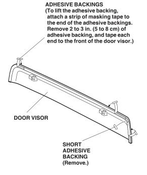
14. Push the two door visor brackets onto the door sash.
