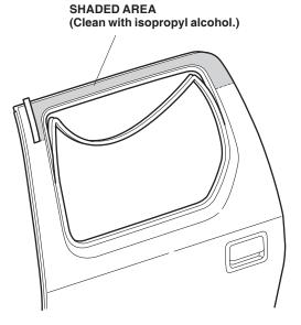
13. Attach a strip of the masking tape to the ends of the long adhesive backings, and remove 2 to 3 in. (5 to 8 cm) of adhesive backings. Fold back the ends, and tape the ends to the front of the door visor. Remove the short adhesive backing.
