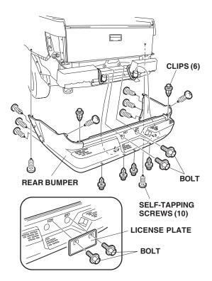
26. On the inside of the rear bumper, locate the six marks. Center punch the six marked locations on the rear bumper. While wearing eye protection, drill a 1 3/16 in. (30 mm) hole through each marked location. First drill with a 3 mm drill bit, and then finish with a 1 3/16 in. (30 mm) holesaw. Remove all burrs from the edges of the holes with a file.
