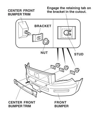
8. While holding light pressure on the trim, carefully remove the adhesive backings from the trim. After removing the adhesive backings, hold the trim firmly against the front bumper with the palm of your hand for 30 seconds.
