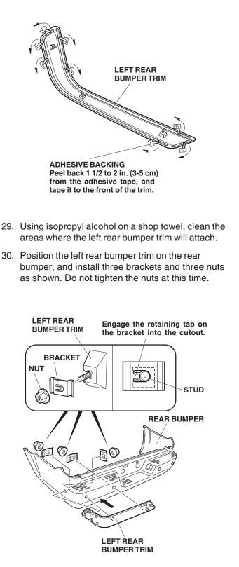
31. Align the upper line of the bumper trim with the masking tape. While holding light pressure on the trim, carefully remove the adhesive backings from the trim. After removing the adhesive backings, hold the trim firmly against the rear bumper with the palm of your hand for 30 seconds.
