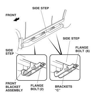
9. Repeat steps 2 through 8 to install the side step on the right side of the vehicle.
