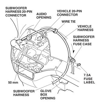
• Route the 5-pin connector side from the subwoofer harness as shown, and secure it to the vehicle harness with four wire ties.
