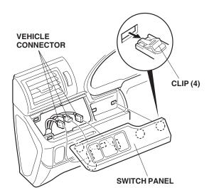
26. Remove the switch lid (two retaining tabs).
