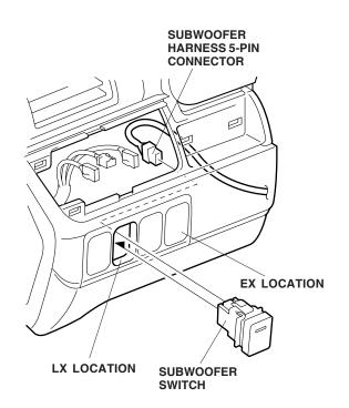
35. Secure the subwoofer harness with two wire ties to the vehicle harness.
