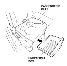
15. If equipped, remove the under seat box bracket (four screws).
