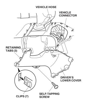
24. Remove the six clips and the three retaining tabs, then remove the instrument side panel.
