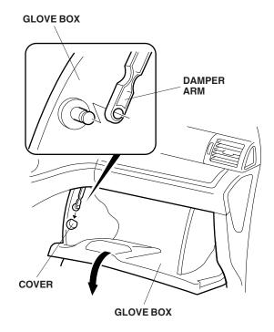
11. Open the glove box, and remove the two stoppers by releasing the two retaining tabs. Remove the two screws that fasten the glove box, and remove the glove box.
