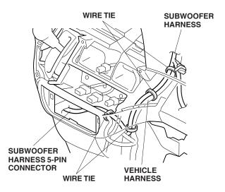
• Secure the subwoofer harness to the vehicle bracket with the three cushion tapes.
