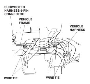
33. Continue routing the 5-pin connector side of the subwoofer harness along the vehicle harness, and secure it to the vehicle frame with two wire ties.
