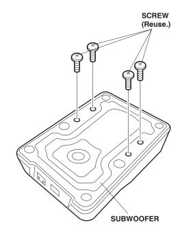
39. Secure the subwoofer to the subwoofer bracket with the four screws you removed.
