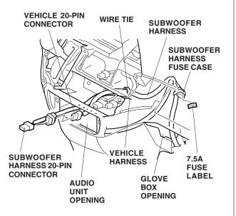
• Route the 5-pin connector side from the subwoofer harness as shown, and secure it to the vehicle harness with four wire ties.
