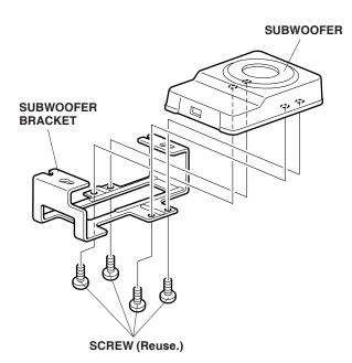
40. Install the subwoofer assembly to the vehicle under the passenger's seat bracket using the bracket four 6 x 12 mm flange bolts.
