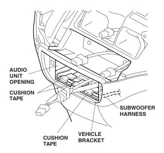
28. Route the 8-pin connector side from the subwoofer harness as shown, and secure it to the vehicle harness with five wire ties.
