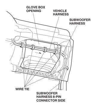
29. Continue routing the 8-pin connector side from the subwoofer harness along the vehicle harness, and secure the harness with four wire ties.
