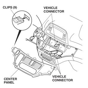
8. Remove the center panel (nine clips and disconnect the connectors).
