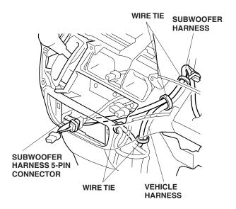
• Secure the subwoofer harness to the vehicle bracket with the three cushion tapes.
