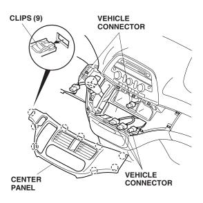
5. Remove the pocket (two bolts, two clips).
