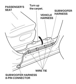
30. Turn up the floor carpet and pull out the 8-pin connector from the subwoofer harness out from under floor carpet opening under the passenger's seat.
