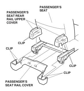
17. Remove the passenger's seat rear rail cover (four clips).
