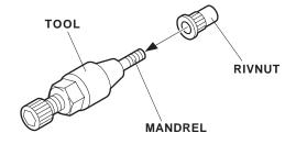
6. Insert the rivnut into the hole in the vehicle panel.
