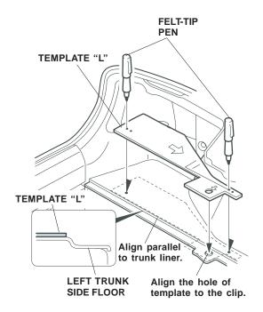
13. Center-punch the marks you made. Lift the trunk liner and check that the center-punched marks you made are centered on the sheet metal rib. While wearing eye protection, drill a 5.5 mm hole through each mark. Start with a 3 mm drill bit and finish with a 5.5 mm drill bit. Remove any burrs, and apply touch-up paint to each hole.
