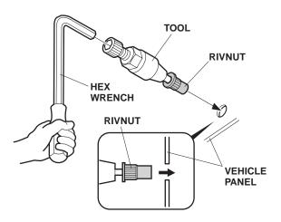
7. While holding the tool with the hex wrench, rotate the 27 mm wrench clockwise and install the rivnut on the vehicle panel.
