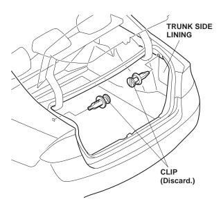
3. While wearing eye protection, drill the two clip holes in the right and left trunk side panels to 9 mm. Remove any burrs, and apply touch-up paint to each hole.
