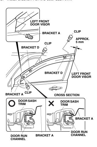
14. Position the left front door visor on the door sash by hooking the front bracket of the door visor on the door sash. Adjust the positions of bracket A and brackets D and install the three clips. Make sure there is no clearance between the bracket and door sash trim. 15. Attach masking tape to the door sash at the ends of the left front door visor, then remove the door visor (three clips).
