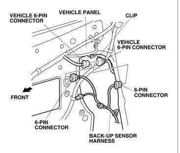
18. Plug the back-up sensor 6-pin connector into the vehicle 6-pin connector. Plug the other vehicle 6-pin connector into the other back-up sensor harness 6-pin connector.
