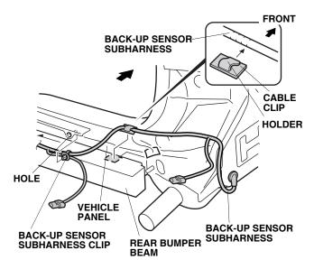
Without Rear Bumper Beam: Install the back-up sensor subharness to the vehicle panel with one wire tie with clip C.
