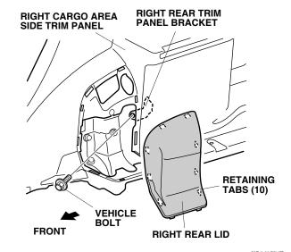
9. Remove the rear door and tailgate weatherstrip from the right cargo area side and two clips from the trim panel.
