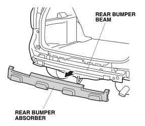
50. Using a utility knife, cut the rear bumper absorber along the preset line at the location shown.
