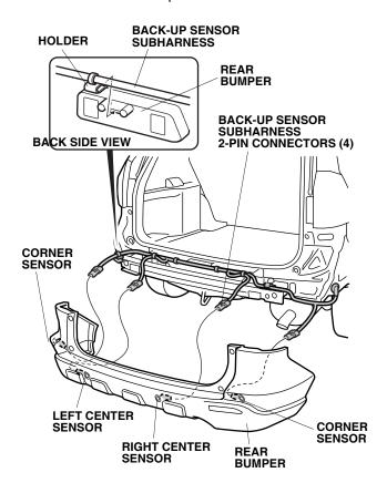
48. Attach the holder of the back-up sensor subharness to the rear bumper as shown.
