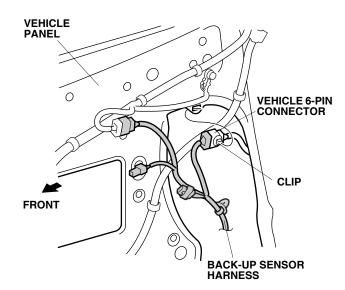
20. Secure the other 6-pin connector to the vehicle harness with one wire tie.
