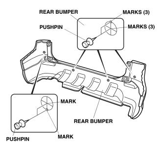
43. While wearing eye protection drill a 3 mm hole at the eight pierced points you just made from the painted side of the rear bumper.
