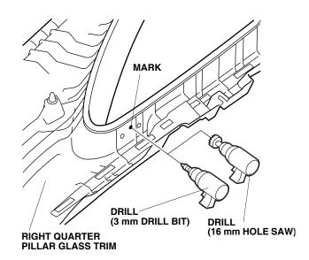
31. Using isopropyl alcohol on a shop towel, clean the right quarter pillar glass trim where the double-sided tape will attach. Remove the adhesive backing from the buzzer. Route the buzzer 2-pin connector through the 16 mm hole, and install the buzzer in the right quarter pillar glass trim with the two self tapping screws. Install with the switch and the volume label toward the front.
