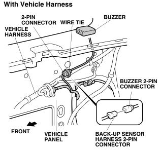
34. Secure the 2-pin connector to the vehicle harness with one wire tie (without vehicle harness: wire tie with clip B).
