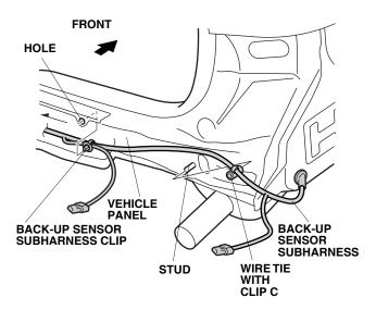
41. Route the back-up sensor subharness as shown and Attach the back-up sensor subharness clips into the holes in the vehicle panel.
