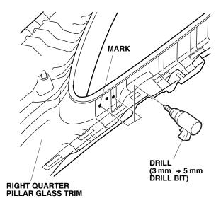
30. While wearing eye protection, drill a 3 mm bit, drill a hole at the marked point, then finish with a 16 mm hole saw. Remove any burrs.
