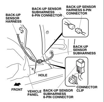
39. Plug the back-up sensor subharness 6-pin connector into the back-up sensor harness 6-pin connector, and install the connector clip into the vehicle panel hole in the area shown. 40. Route the back-up sensor subharness as shown, and install the back-up sensor subharness clip into the vehicle panel hole. Secure the back-up sensor subharness:
