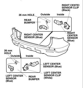
47. With the help of an assistant bring the rear bumper near the vehicle, plug in the four back-up sensor subharness 2-pin connectors into the sensors, and reinstall the rear bumper.
