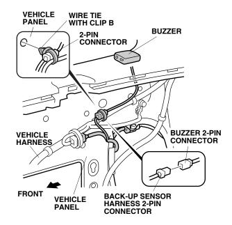
35. Secure the buzzer harness to the vehicle harness with one wire tie.
