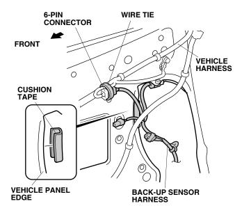
21. Using isopropyl alcohol on a shop towel, thoroughly clean the area where the cushion tape will attach. Attach the cushion tape to the edge of the vehicle panel at the location shown.
