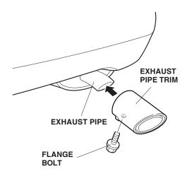
2. With the flange bolt on the bottom, facing down, slide the exhaust pipe trim onto the exhaust pipe until it bottoms.
