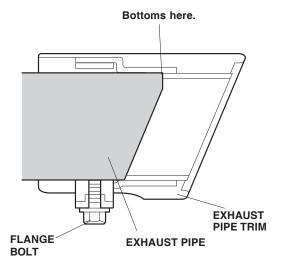
3. While pushing the exhaust pipe trim firmly against the exhaust pipe, tighten the flange bolt. Torque to 10 N·m (7 lb-ft).
