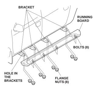
Align the rear of the running board with the end of the inner fender, then tighten the flange bolts you installed in step 9. Torque 14 flange bolts to 27 N·m (20 lbf·ft) and the one remaining flange bolt to 7 N·m (5 lbf·ft).
