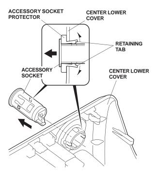
8. Remove the accessory socket protector from the dashboard center lower cover by releasing the two retaining tabs.
