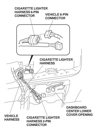
Connect the vehicle 2-pin connector and cigarette lighter harness 2-pin connector into the socket of the cigarette lighter. Reinstall the dashboard center lower cover.
