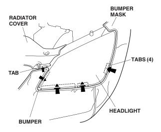
9. Insert the six tabs between the grille and the bumper.
