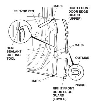
4. Position the hem sealant cutting tool against the door edge, and trim the seam sealant from mark to mark, top and bottom.
