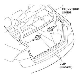
3. While wearing eye protection, drill the two clip holes in the right and left trunk side panels to 9 mm. Remove any burrs, and apply touch-up paint to each hole.
