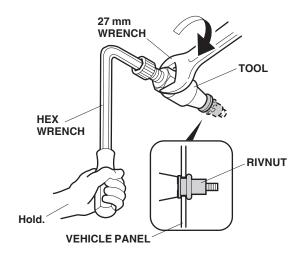
8. Remove the tool from the rivnut by turning the hex wrench counterclockwise.
