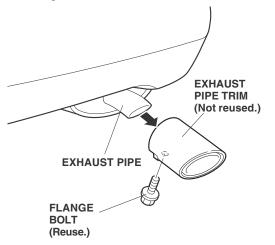
2. Partially thread flange bolt into the exhaust pipe trim.
