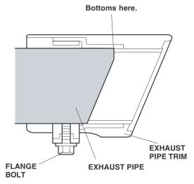
While pushing the exhaust pipe trim firmly against the exhaust pipe, tighten the flange bolt. Torque to 10 N·m (7 lb-ft).
