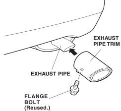
3. With the flange bolt on the bottom, facing down, slide the exhaust pipe trim onto the exhaust pipe until it bottoms.
