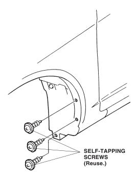
4. Position the splash guard on the inner fender, and install the three self-tapping screws you removed. Tighten the three self-tapping screws in the order shown.
