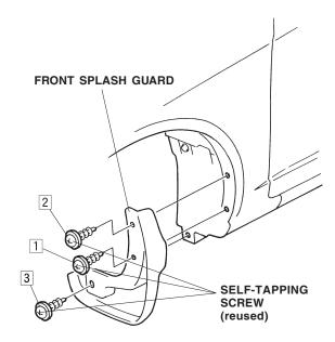
5. Turn the steering wheel all the way clockwise, and repeat steps 3 and 4 to install the right front splash guard.
