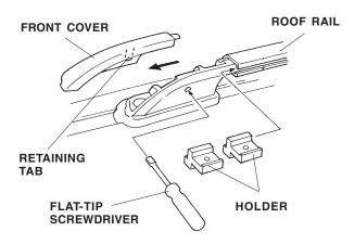
2. Insert two holders in the groove of the roof rail.
